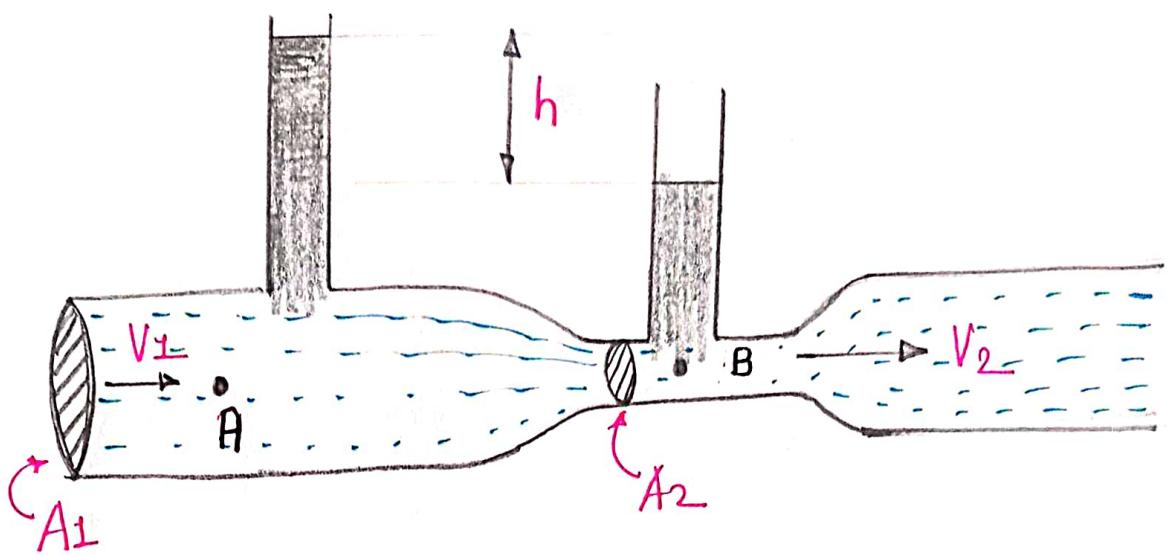
The venturi-tube is a device which is used to measure the flow speed of incompressible fluid.
